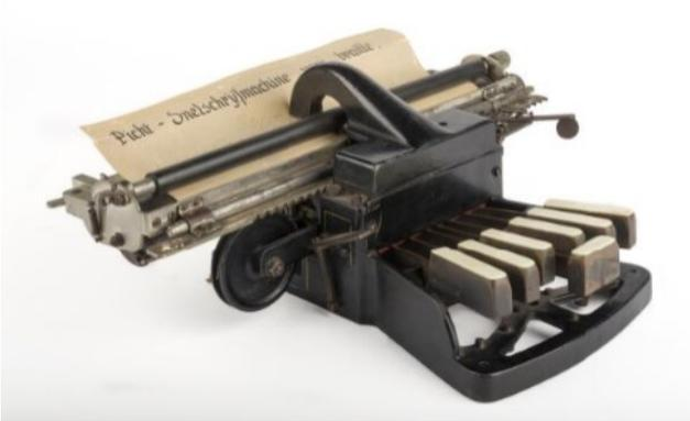
*An example of the aid-collection; the 'Picht' typewriter. The machine has a keyboard of six keys and a space key. By tapping one or more keys simultaneously, dots (letters in braille) are pressed into the paper.*
